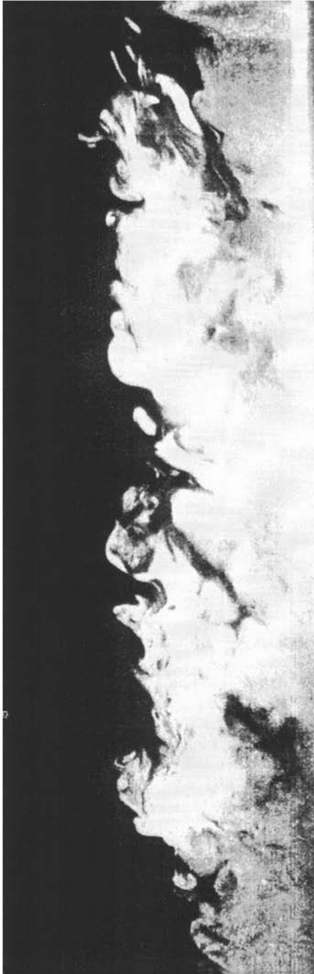
Figure 33 Characteristic turbulent flow near a boundary. With permission of the American Institute of Physics.
